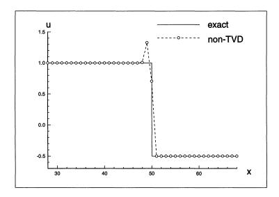
FIGURE 1. Second order TVD MUSCL spatial discretization. Solution after 500 time steps. Top: TVD time discretization (2.4); Bottom: non-TVD time discretization (2.5).
